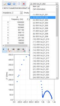
b) Seelect Impedance, Z in polar, Admittance, Y in Polar, Modulus, M in polar, Dielectric Constant, E in polar. (in polar = in Polar Coordinate)
