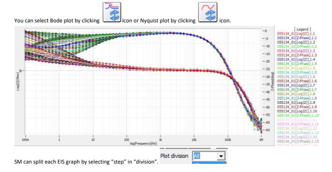
You can split data by file, cycle or step. Splitted data set's color was changed and graph line will be broken
