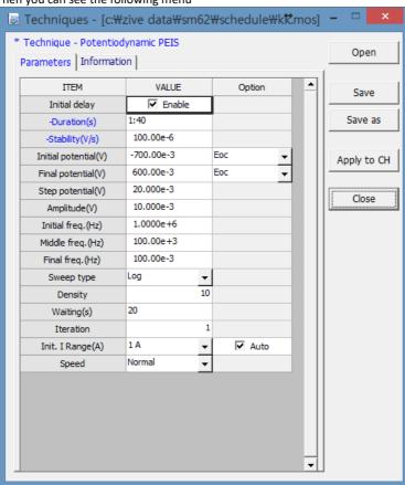
4. Select Frequency scanning potentiodynamic PEIS at left technique selection region. The parameter editing region is located at right. Input figure for parameter setting as the follows..
