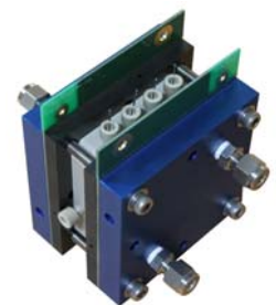
MCC with fuel cell hardware fixture
